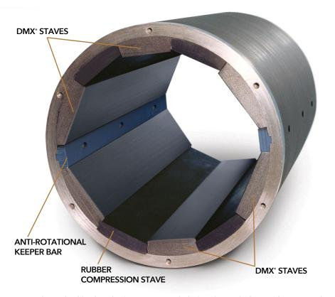
DMX\* Advanced Rubber-based Polymer Staves are locked in place in the housing by a patented rubber stave system. When the rubber staves are compressed by the compression head, they expand outward locking the adjacent DMX\* stave bearings in place.
