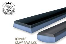
Specially formulated proprietary nitrile rubber water-lubricated staves have a 15 to 20 glass-smooth finish and 80 Durometer, Shore A hardness, backed by a light-weight polymer corrosion resistant ultra-high molecular weight polymer alloy backing. It delivers unbelievably low friction at extremely low journal velocities. Available in radius back and dovetail stave designs.
