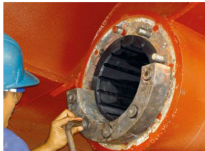
Tightening the outer collar compresses the staves and will adjust the internal diameter to the exact clearance
