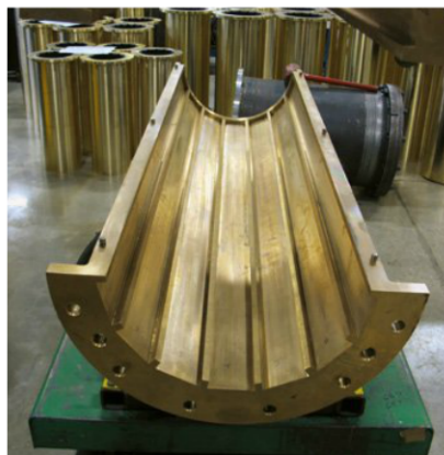
A dovetail housing fully machined ready for the dovetailed rubber staves
