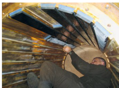
Fitting staves to a Russian ice-breaker's sterntube
